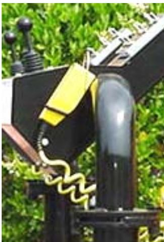
1. Place the handset into the cradle at the operator's station. Route cable over the resting bolt.
