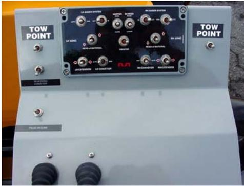
When activated, after the ignition switch has been turned to the "ON" position, this switch will engage the Pave Resume feature, (see section 15.0 explaining Pave Resume operation), and the light will stop flashing. When activated again the paver will return to pause mode and the pause light will start flashing. When in pause mode the yellow pause light will flash, confirming that the steering controls are disabled.
