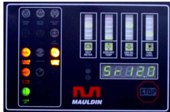
Activate the DISPLAY TOGGLE one more time and the LED on the control panel reads "SR 12.0". This stands for sonic **S**etting **R**ight. All functions are identical to the above information regarding "**SL**".
