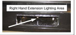
With extension burners operating, turn on gas to main screed burners and point hand lighting torch at the lighting area.
