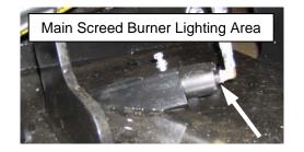
$\ensuremath{\text{VERY IMPORTANT}}$  – First light the inboard burners, then light the outboard burners.
